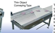
The conveyed objects coming in a scattered condition are lined up in a row on one side.
